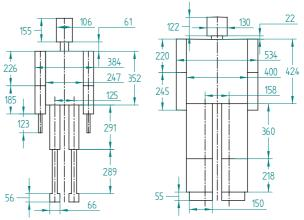
Figure 2: The proportions of typical human anatomy compared to the matching proportions of GuRoo's anatomy. The dimensions indicate the sizes for a human scaled to 1.2m in height.
