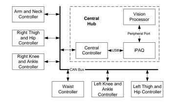
Figure 4: Block diagram of the distributed control system.
