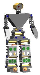
Figure 1: Full CAD model of the GuRoo humanoid robot.
